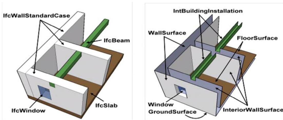
Figure 2. Comparison between IFC (left) and 3D GIS (right) geometry modelling paradigms (van Berlo & de Laat, 2010)
