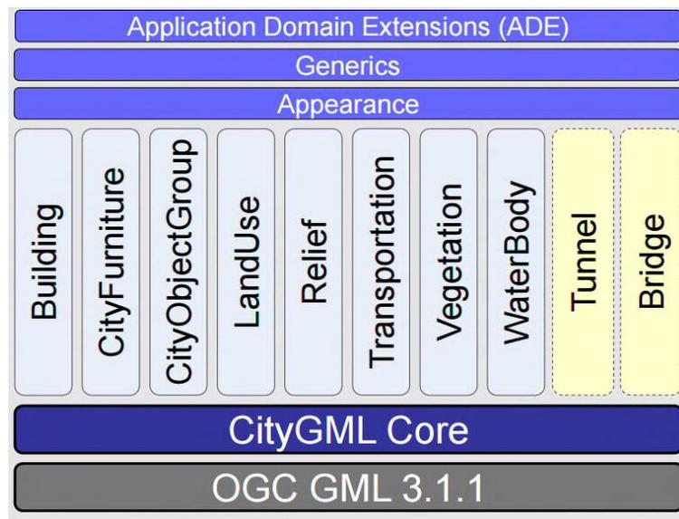
Figure 1. Modular Structure of CityGML (Kolbe & Nagel, 2011)
